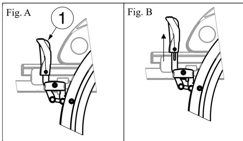
To apply the brakes (Fig A):
