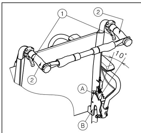
1. Pull the lever ① on both sides towards the push handle ② to adjust the backrest.
