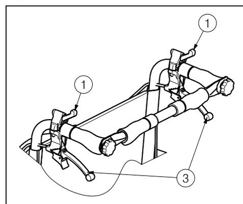
If your wheelchair features drum brakes, the handles ③ are used as brakes.
