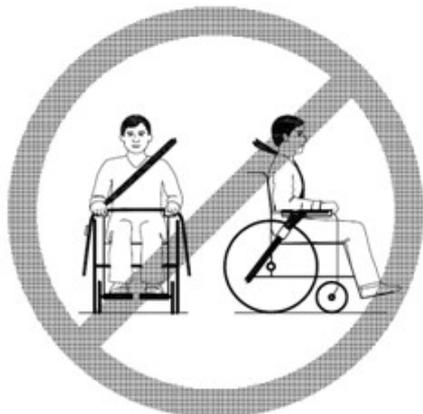
PELVIC RESTRAINTS SHOULD MAKE FULL CONTACT ACROSS THE FRONT OF THE BODY NEAR THE JUNCTION OF THE THIGH AND PELVIS
